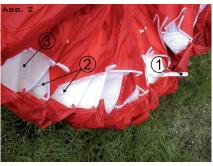
Press each reinforcement neatly onto the next. That will make for a strong packing that is protected from bending.
