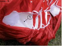
That's what the finished glider looks like. Now the back part can be folded rail by rail and rolled up.
